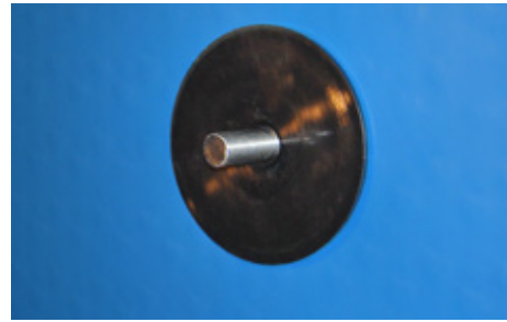
Figure 34: BA-anchor during curing
